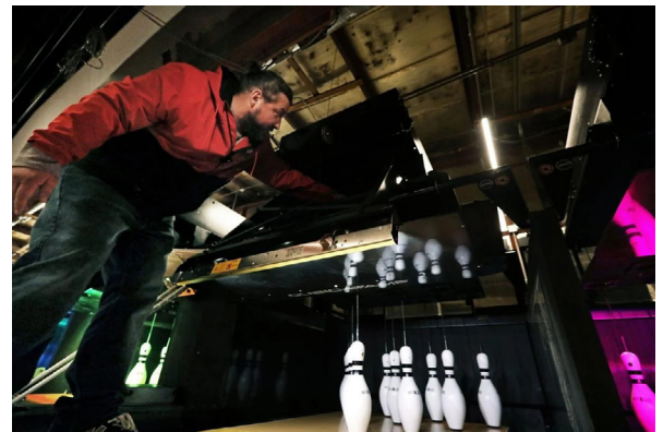
Eddie Bryant, general manager at the 300 Club in Green Lake, shows the inner workings of one of 12 string pin-setting machines at the bowling center. - AMBER ARNOLD, STATE JOURNAL
