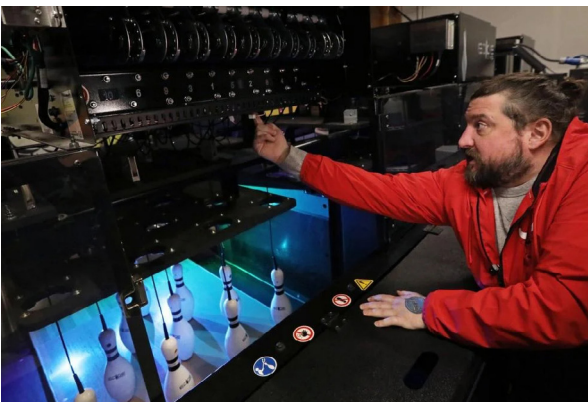
Eddie Bryant, general manager at the 300 Club, shows how tension on strings can be adjusted. Bryant said tangles are uncommon and easier to fix than a jammed pin in a traditional pin setting machine. AMBER ARNOLD, STATE JOURNAL
